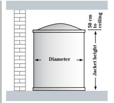
minimum wall clearance is prescribed for double-walled tanks.
